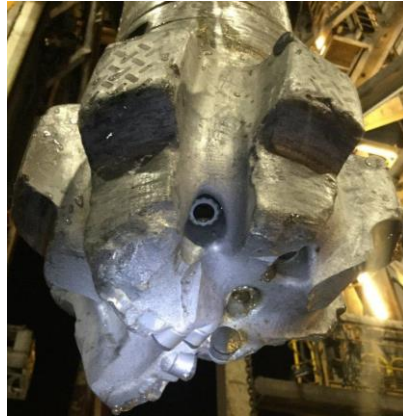
Figure 3. Broken blade on Polycrystalline Diamond Compact (PDC) bit due to backward whirl
