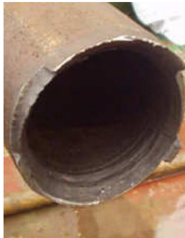
Figure 4. Twist off in 3½-in. drill pipe
