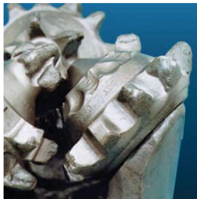
Figure 2. Broken teeth due to axial vibration.
